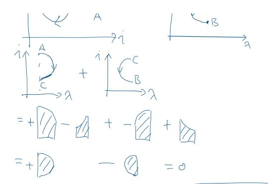
Sectro magnet!  $L(x) = \frac{N^2}{R(x)}, R(x) = \frac{x}{u_0 A},$   $W_m = \frac{1}{2}L(x)i^2 = \frac{i^2}{2} \frac{u_0 A N^2}{x}$   $f = 4 \frac{dW_m}{dx} = -\frac{1}{2} \frac{u_0 A N^2}{x^2} \quad (increasing x)$
