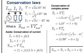
$$\begin{split} S_1 &= VI_1 \\ &= (\sqrt{2} \angle 45^\circ) \left(\frac{1}{\sqrt{2}} \angle 45^\circ\right)^* \\ &= 1 \angle 0^\circ = 1 + 0j \\ \overline{S}_2 &= \overline{VI}_2^* \\ &= (\sqrt{2} \angle 45^\circ) \left(\sqrt{2} \angle - 45^\circ\right)^* \\ &= 2 \angle 90^\circ = 0 + 2j \end{split}$$
