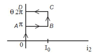
The machine is operated over the cycle ABCD while  $i_1 = I_0$ . Find the energy converted from electrical to mechanical
