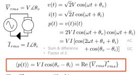
$$\overline{V}_{rms}\overline{I}_{rms}^* = (VI)e^{j(\theta_v - \theta_i)}$$
