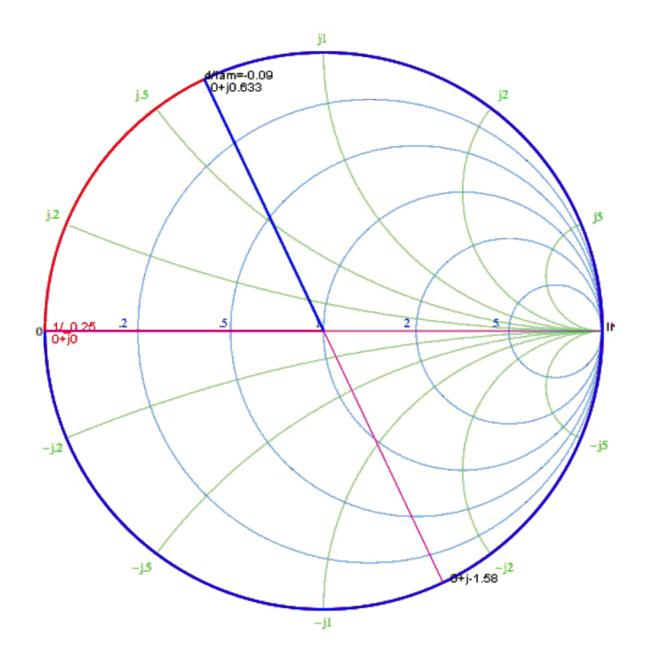
(b) (4 points) The procedure is the same as that in (a), except that now  $Z_{os} = 100 \,\Omega = 2Z_o$ , or  $Y_{os} = 0.5Y_o$ . For this case, we still find that  $y(d_1) = 1 + j1.58$ , or  $Y(d_1) = \frac{1}{Z_o}(1 + j1.58)$ . Thus, the stub admittance should be  $Y_s = \frac{1}{Z_0}(-j1.58) = \frac{1}{Z_{OS}}(-j3.16) = -j3.16Y_{os}$ , or  $y_s = -j3.16$ . By rotating from the short point to the ys point, we obtain  $d_s = 0.049\lambda$ .
