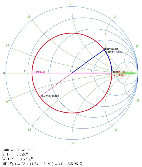
(b) (2 points) At the generator end (source plane, source port, input port, etc), the generator sees nothing but two lumped elements with impedance  $50 \Omega$  and  $41 + j45.25 \Omega$ . A simple voltage dividing rule gives:
