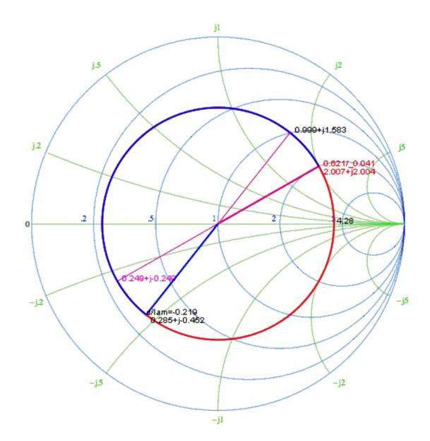
To determine the length of the stub, we locate the short point  $y = \infty$  and rotate towards the generator (clockwise) until we reach the point y = -j1.58. The rotation distance is the length of the stub:  $d_s = 0.09\lambda$
