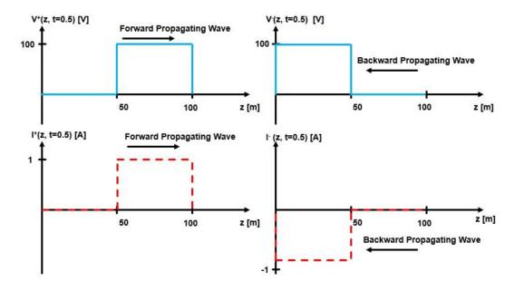
Combining the waveforms we get the voltage and current as below.
