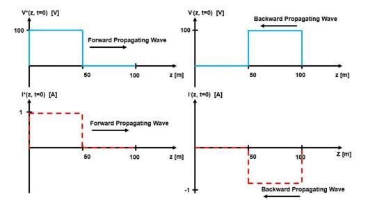
Since the wave travels at 100  $\frac{\rm m}{\mu \rm s},$  after 0.5  $\mu \rm s$  the wave have traveled 50 m and have the following waveform.
