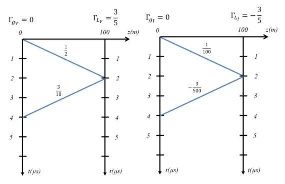
Voltage (left) and current (right) bounce diagrams for voltage source  $f(t) = \delta(t)$ . The expressions of V(z, t) and I(z, t) are given by
