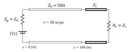
The equivalent impedance seen at z = 100 m looking from the source is  $Z_1$ . If no reflection at z = 100 m is desired, the equivalent impedance must be as same as that of the transmission line, hence  $Z_1 = Z_0 = 50 \Omega$ .
