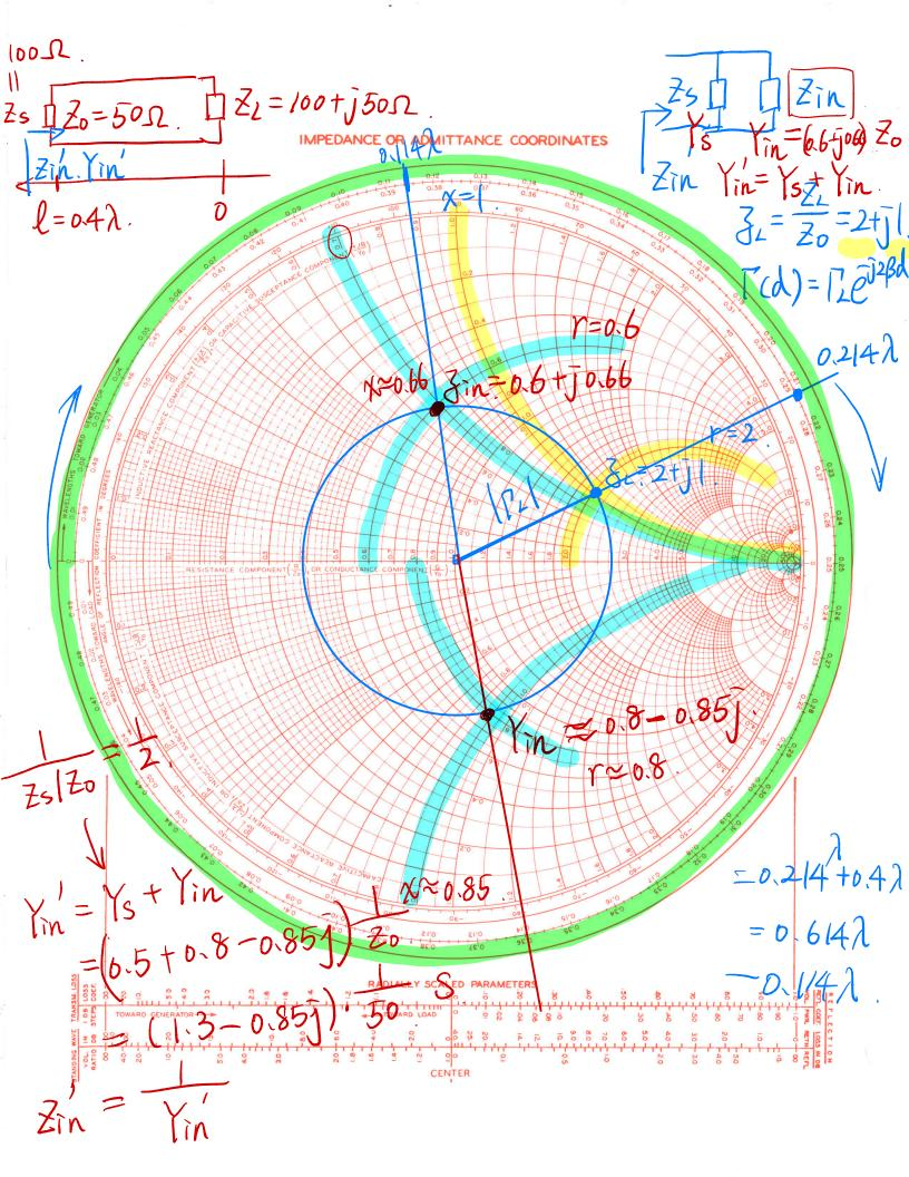
**Example 2:** The TL network described in Example 1 is connected to a generator with open circuit voltage phasor  $V_g = 100 \angle 0$  V and internal impedance  $Z_g = 25 \Omega$ . What is the average power (a) input of the shunted line, (b) delivered to the shunt element, delivered to the load.
