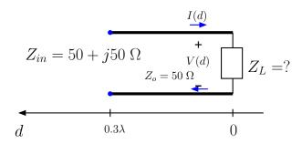
**Example 3:** A TL of length  $l=0.3\lambda$  has an input impedance  $Z_{in}=50+j50\,\Omega$ . Determine the load impedance  $Z_L=Z(0)$  and  $Y_L=Y(0)$  given that  $Z_o=50\,\Omega$  for the line.
