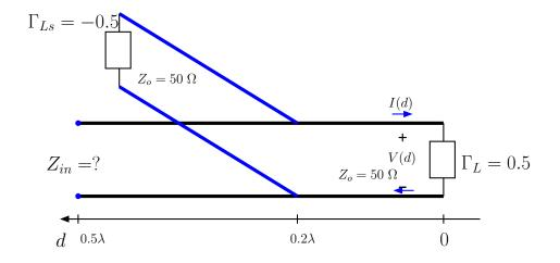
**Example 4:** A TL of length  $l = 0.5\lambda$  and  $Z_o = 50 \Omega$  has a load reflection coefficient  $\Gamma_L = 0.5$  and and a shunt connected TL at  $d = 0.2\lambda$ . The shunt connected TL has  $l = 0.3\lambda$ ,  $Z_o = 50 \Omega$ , and a load reflection coefficient  $\Gamma_L = -0.5$ . Determine the input impedance of the line.
