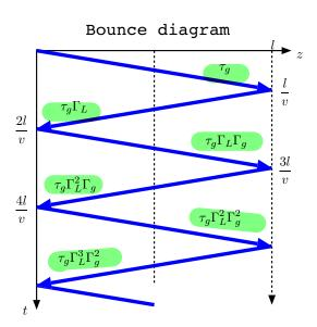
• Although these series formulae<sup>1</sup> look daunting, only the lower order terms usually matter — that is true because  $|\Gamma_L| \leq 1$  and  $|\Gamma_g| \leq 1$  and thus  $(\Gamma_L \Gamma_g)^n$  is typically a rapidly diminishing function of n (unless the ckt is "dissipation free" and resonant, a concept explored in Lecture 31).
