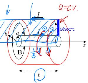
Shorted coax circulates a current I linking a magnetic flux  $\Psi$  confined to a region bounded by the outer conductor of the coax.
