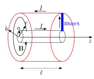
Shorted coax circulates a current I linking a magnetic flux  $\Psi$  confined to a region bounded by the outer conductor of the coax.
