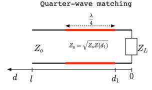
Consider a TL with  $Z_L = 100 - j50 \Omega$  and  $R_g = Z_o = 50 \Omega$ . Since  $Z_L \neq Z_o$ , the load is unmatched and the VSWR>1.
