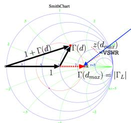
Since  $\Gamma(d_{max}) = |\Gamma_L|$  (reflection coefficient at  $d_{max}$  location is the radius of red circle  $|\Gamma_L|$ .
