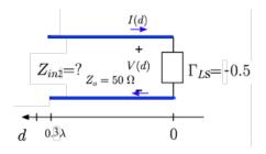
Step 3: Black TL with length  $l=0.3 \lambda$  and  $Z_o=50 \Omega$ , at load side it has parallel impedance  $Z_{in1}$  and  $Z_{in2}$ , find input impedance  $Z_{in}$
