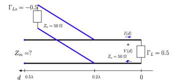
Step 1: Black TL with length l=0.2  $\lambda$  and  $Z_o=50$   $\Omega$ , load reflection coefficient  $\Gamma_L=0.5$ , find input impedance  $Z_{in1}$  at l=0.2  $\lambda$ .
