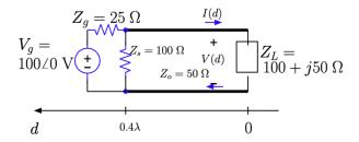
a) Average power  $P_{in}$  at the input of the shunted line
