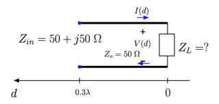
$\circ$  From input impedance  $Z_{in}$  to load impedance  $Z_L$
