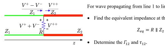
For wave propagating from line 1 to line 2
