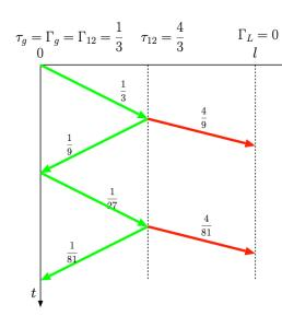
Draw its bounce diagram. Notice that in line 1, we have both forward and backward traveling waves (two green arrows), while in line 2, there's only forward traveling wave (red arrow), since  $\Gamma_L = 0$ .
