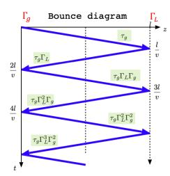
Compile with the three coefficients  $\tau_g$ ,  $\Gamma_L$ , and  $\Gamma_g$ , together with the green font magnitude for the waves in the bounce diagram, we can write the V(z,t) at the midpoint of the TL as
