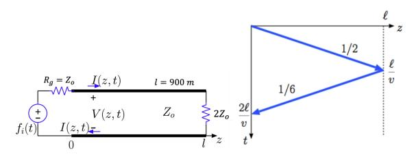
The TL has matched impedance at the source end  $R_g = Z_o$ , so  $\Gamma_g = 0$ .
