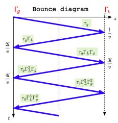
A convenient tool for understanding TL transients is a bounce diagram. The horizontal axis of the diagram is the z coordinate, and the downward axis is time t.
