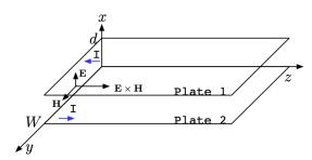
In a parallel-plate transmission line, we assume that TEM wave fields in between the TL are
