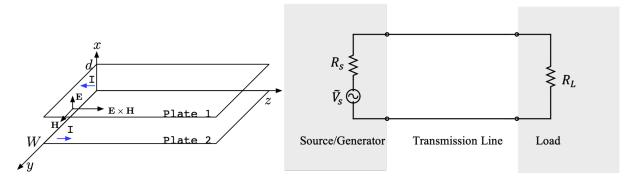
In general, we can excite the transmission line using a Thevenin or Norton circuit on the source/generator end, and terminate the transmission line with any resister, inductor, or capacitor on the load end.
