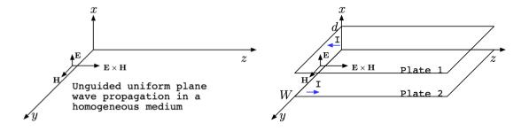
Then it will introduce positive charges on the upper surface of bottom plate, and negative charges on the bottom surface of top plate (two inner surfaces), so that the electric field is pointing from positive charges to negative charges (in the +x direction).
