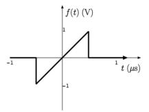
Consider an  $\hat{x}$ -polarized plane TEM wave field in free space  $\vec{E}(z,t) = \hat{x}f\left(t - \frac{z}{c}\right)$ , where  $f(t) = 2t \, \mathrm{rect}\left(\frac{t}{1us}\right)$ , draw the time plot and position plot of  $\vec{E}$  field.
