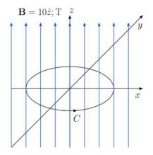
A conducting loop of a radius r = 0.1 m (see figure in the margin) is being rotated about the x axis with frequency of  $f = \omega/2\pi = 60$  Hz in a region with a DC magnetic field of  $B = 10\hat{z}$  T. Determine the induced current in the loop if the loop resistance is 12  $\Omega$ .
