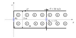
A conducting bar of resistance  $R_1 = 1 \Omega$  ohms is moved in the x-direction with a velocity v = $3\hat{x}$  m/s on a pair of perfect conducting (R = 0)stationary rails 2 m apart terminated with a load x resistance  $R_2$  at x = 0, all constituting a rectangular contour C to be taken counterclockwise. A constant magnetic field of  $B = 1\hat{y} T$  is linked through contour C.
