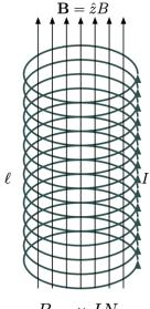
Consider a long solenoid with length l, cross-sectional area A, and a density of N loops per unit length.
