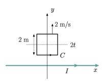
Consider the magnetic flux density  $\vec{B} = \frac{\mu_o I}{2\pi r} \hat{\phi}$  produced by current *I* flowing along the x axis. What is the EMF  $\mathcal{E}$  of a square loop *C* of area 4  $m^2$  moving on xy-plane with edges parallel to x-and y-axes, if its center is located at y=2t m as a function of time?
