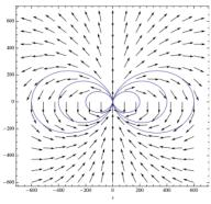
The far field structure of the magnetic field a loop is the same as the far field pattern of the electric field of a dipole.
