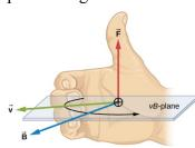
**Right hand rule**: point your right thumb in the direction of current flow; your fingers will point in direction  $\hat{\phi}$ .
