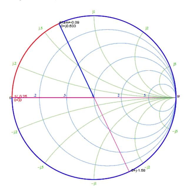
(b) (4 points) The procedure is the same as that in (a), except that now  $Z_{os} = 100 \Omega = 2Z_o$ , or  $Y_{os} = 0.5Y_o$ . For this case, we still find that  $y(d_1) = 1 + j1.58$ , or  $Y(d_1) = \frac{1}{Z_o}(1 + j1.58)$ . Thus, the stub admittance should be  $Y_s = \frac{1}{Z_o}(-j1.58) = \frac{1}{Z_{OS}}(-j3.16) = -j3.16Y_{os}$ , or  $y_s = -j3.16$ . By rotating from the short point to the ys point, we obtain  $d_s = 0.049\lambda$ .
