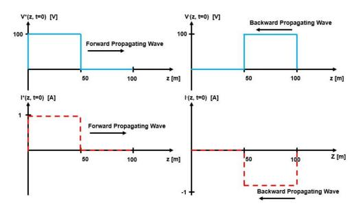
Since the wave travels at  $100 \, \frac{\text{m}}{\mu \text{s}}$ , after  $0.5 \, \mu \text{s}$  the wave have traveled 50 m and have the following waveform.
