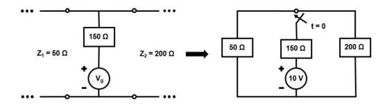
this configuration the voltage boundary conditions dictate that  $V = V_g - R_g I$ ,  $V = Z_1 I$ , and  $V = Z_2 I$ . The currents must have the relation  $I = I_1 + I_2$  if I is the current flowing from the source,  $I_1$  and  $I_2$  are the currents flowing into each transmission line. These constraints are exactly the same as a circuit with the same source configuration connected to two parallel resistors. This greatly simplifies finding the injection coefficient. Now
