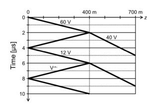
The impedance and transmission time of line 1 are  $Z_1$  and  $T_1$  and those of line 2 are  $Z_2$  and  $T_2$ . Using the figures, identify the following parameters in appropriate units:
