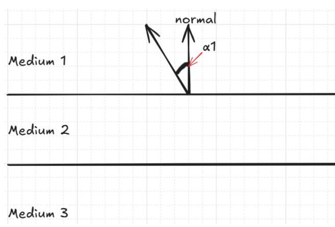
It is stated that the boundaries between the media are charge-free, and that medium 2 is now a slab of finite thickness, while medium 3 is free space. To find  $\alpha_3$ , the angle from normal of the electric field in medium 3, we must again use boundary conditions.
