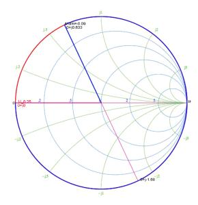
b) The procedure is the same as that in (a), except that now  $Z_{os} = 100(\Omega) = 2Z_o$ , or  $Y_{os} = 0.5Y_o$ . For this case, we still find that  $y(d_1) = 1 + j1.58$ , or  $Y(d_1) = \frac{1}{Z_o}(1 + j1.58)$ . Thus, the stub admittance should be  $Y_s = \frac{1}{Z_o}(-j1.58) = \frac{1}{Z_{OS}}(-j3.16) = -j3.16Y_{os}$ , or  $y_s = -j3.16$ . By rotating from the short point to the ys point, we obtain  $d_s = 0.049\lambda$ .
