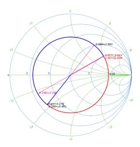
To determine the length of the stub, we locate the short point  $y = \infty$  and rotate towards the generator (clockwise) until we reach the point y = -j1.58. The rotation distance is the length of the stub:  $d_s = 0.09\lambda$
