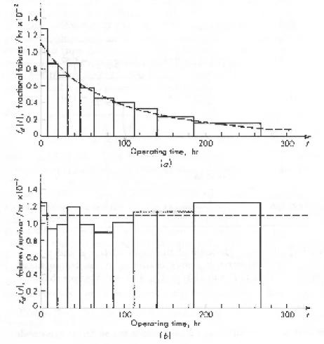
Failure Density and Hazard Rate for the Given Data
