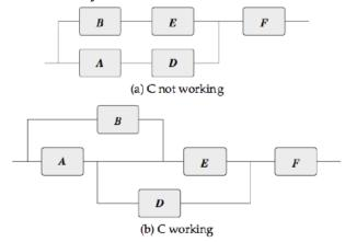
The part (a) is already of the series/parallel system, whereas part b needs further dividing around node E. Note that part b should not be viewed as a parallel connection of A and B, connected serially to D and E in parallel; such a diagram will have the path BCDF, which is not a valid path in the original system.
