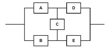
Use the conditional probabilities to determine an expression for the system reliability as a function of component reliabilities. Assume that the reliability of each component is equal to *R*. **Hint:** Try to find a node around which you can simplify the analysis.
