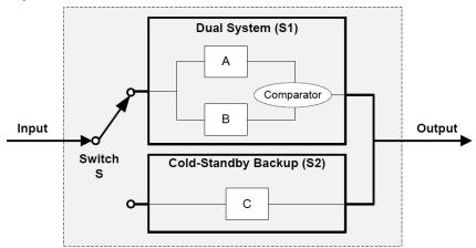
Assume that A and B are identical components and the switching circuit S and the comparator are perfect. We model the lifetime of the components A, B, and C with three independent random variables  $X_1$ ,  $X_2$ , and  $X_3$  Assume  $X_1$  and  $X_2$  are exponentially distributed with parameter  $\lambda$  and  $X_3$  is exponentially distributed with parameter  $3\lambda$ .
