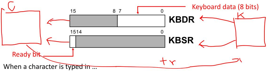
1. Its ASCII code is placed in bits [7:0] of KBDR (bits [15:8] are always zero)
