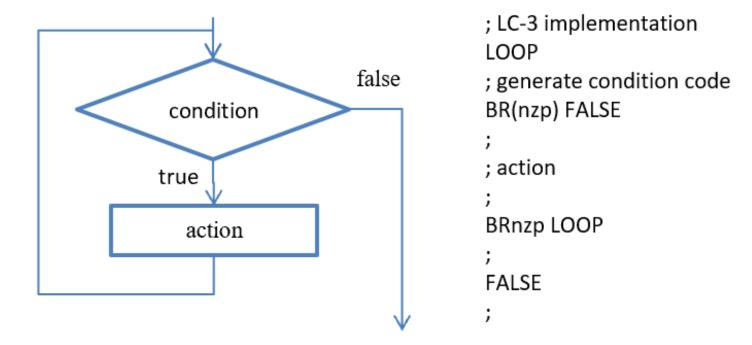
Such construct implements a loop structure in which *action* is executed multiple times, as long as some *condition* is true
