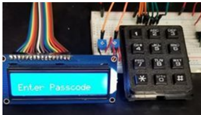
Figure 4: LCD prompts user and displays keypad input.
