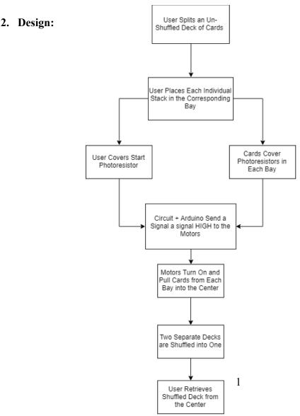
The goal of our contraption is to shuffle two stacks of cards together. This task is accomplished first by the user manually splitting the deck in half and placing each half in separate bays. Once the cards are placed into separate bays, the user covers the shuffle photoresistors. Covering the shuffle photoresistors after loading the bays should turn on each motor. The motors should toss the two individuals decks into each other in the center thus producing one shuffled deck in the center.
