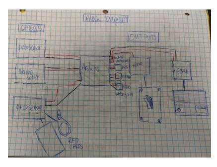
This is the block diagram. As you can see, all of the inputs and outputs are connected to the Arduino. Included in the block diagram is also how each of the parts is connected to the real world, represented by the blue line instead of the red and black lines.
