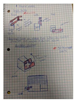
On the top is the light switch servo, which I have mostly done in CAD, but not to the point where it is able to be 3D printed. On the bottom is the AC button pusher, which I just have made out of cardboard.
