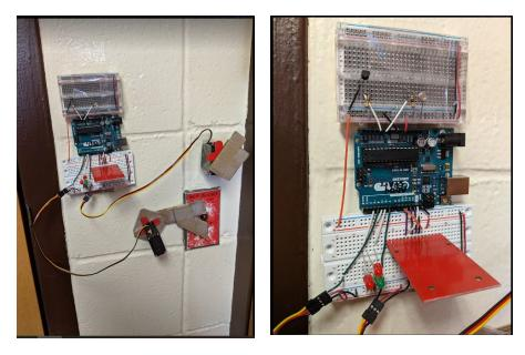
Pictured on the left is the whole system attached to the wall. I did not make the servo mounts out of cardboard, so that is why the servo is backward. One thing that is wrong about the cardboard diagram is that the part that actually flips is shaped like a y, with one part slanty. The slanty part does less work on the light switch because
