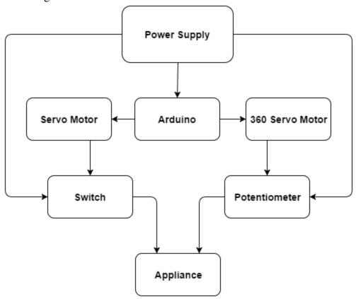
Power Supply: 110v wall outlet for switches, 9v battery for arduino
