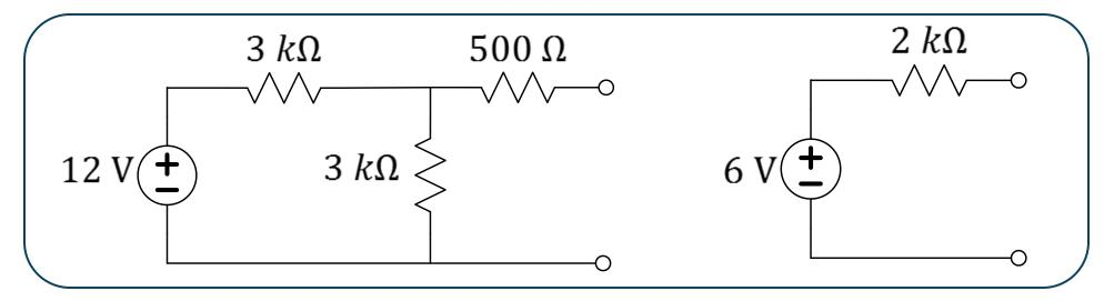
Q: If both circuits produce the same I = mV + b plot, can the IV data be used to tell which of the two circuits is "in the box"?
