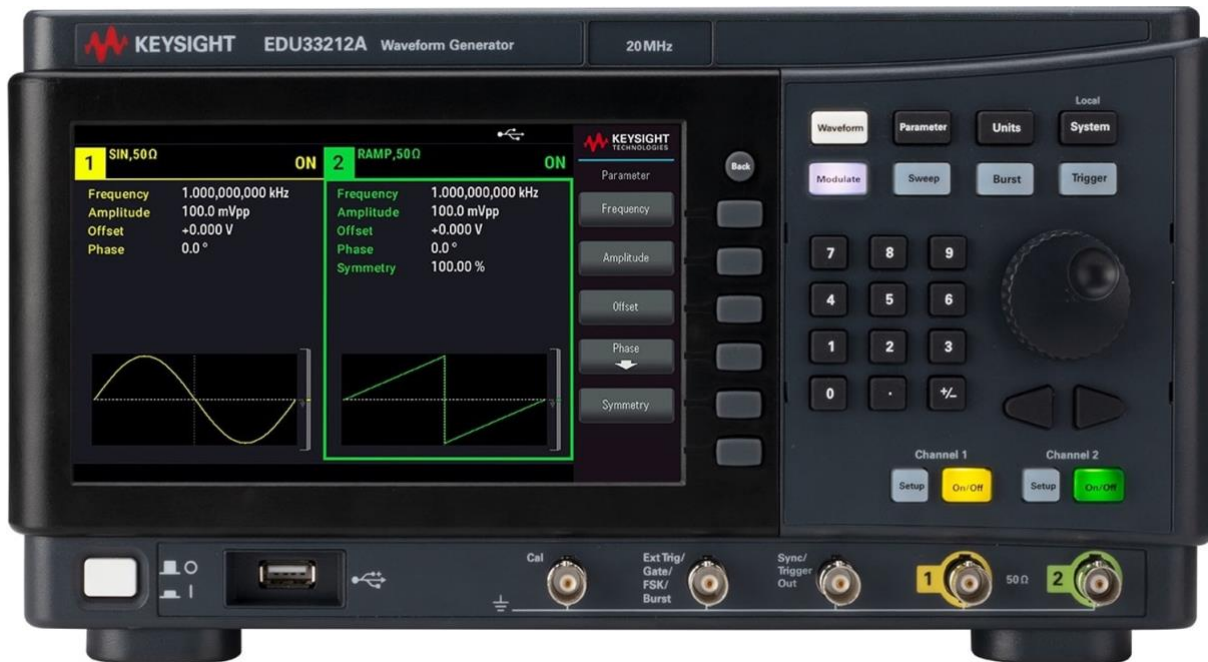
Figure 2: The front panel of the Keysight EDU33212A function generator. At the BNC output, the center pin is the positive voltage reference while the outer shield is the negative (often the “ground” reference).
