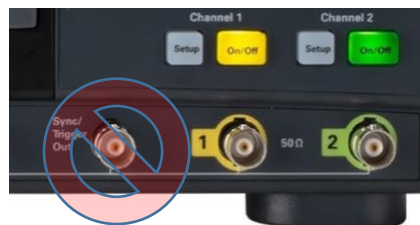
Figure 3: We will never use the SYNC port in ECE 110. Please do not mistake it for the OUTPUT port!
