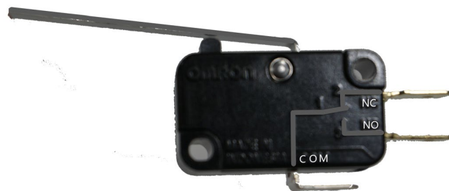
Figure 2: The snap-action (lever) switch.
