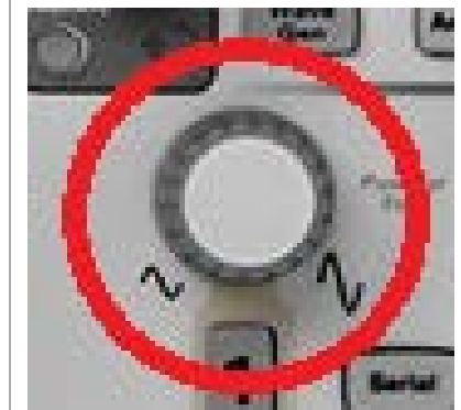
Figure 8: Adjust the view using the vertical scale adjust (visible height of the signal) and the horizontal scale adjust (amount of time shown on the screen).
