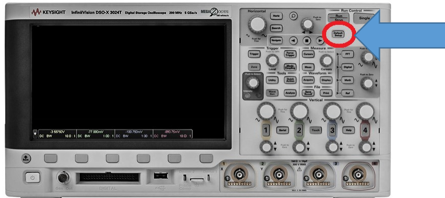
Figure 4: The oscilloscope's Default Setting.
