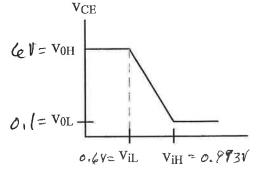
$$U_{OL} = V_{CESAT} = 0.1V$$
