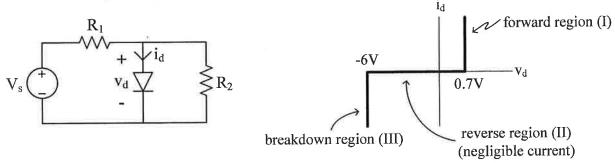
(a) (5 pts) Complete each of the circuit models below by inserting in place of the diode the linear model appropriate for the specified region of operation, for example, resistor, open or short circuit, voltage or current source and its value.
