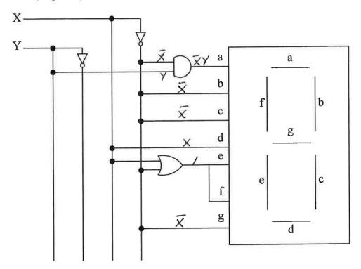
Complete the table below. Hint: To save time, first write a Boolean expression for each of the 7 segments.  $a = \overline{x}y$ ;  $b = c = \overline{x}$ ; d = x; e = F = 1,  $g = \overline{y}$
