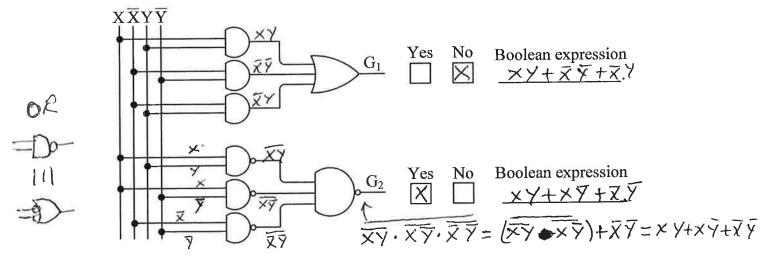
(c) (3 pts) The optimal circuit for G is shown below. Circle the unknown gate.
