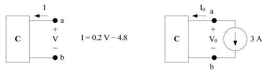
(a) (4 pts) Component  $\bf C$  is connected to an ideal current source shown on the right above. Determine  $\bf V_0$ .
