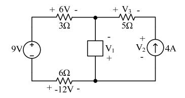
(a) (8 pts) Write a KVL equation involving  $V_1$  as the only unknown and then solve for  $V_1$ .
