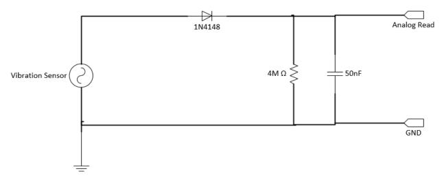
(4M Ohmn can be built by 4 1M Ohmn resistors in serious and 50nF can be built by 2 100nF capacitors in serious).
