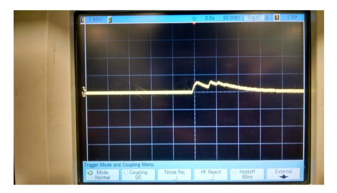
You are recommended to write a code that triggers when the reading exceeds a certain threshold and holds the largest value for 20-100 loop() executions (save the largest value in a global variable for 20 to 100 loop() iterations, during the iteration, replace the variable and zero the iteration counter if a larger value is detected). This should be able to pick up the peak reading from the sensor. It should also filter out the low amplitude oscillations.
