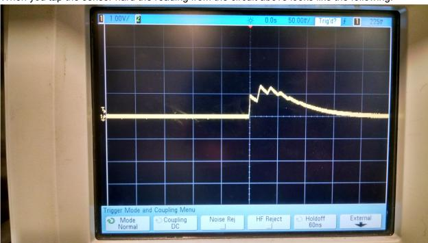
When you tap it lighter, the settling time is similar and the peak amplitude drops:
