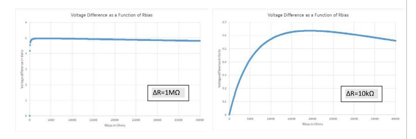
As you can see when the resistance changes over a large range the value of  $R_{bias}$  is almost irrelevant. The voltage V varies across nearly 5V for the range of resistance values in your resistor kit. In this case you have the luxury of taking into account the power consumption in the resistors. In this case you can choose a resistor with a higher value so that the current flowing through the voltage divider is minimized ensuring that not much power is wasted.
