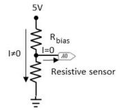
To choose the proper resistance let's look to Excel to help us. The two graphs below show the range of the voltage labeled V in the schematics for the case where the range of the resistances of the sensor is really large (like the photo-resistor) and the range of resistances is not as large (like the flex-sensor).
