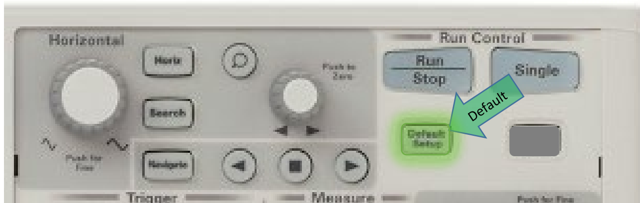
Figure 3: Always start by pressing the Default Setup on the oscilloscope.
