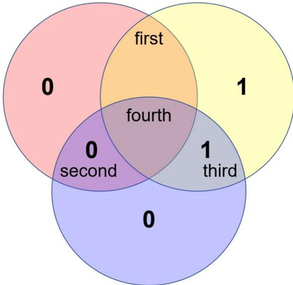
The "fourth" bit of the message must be 1 in order to have two 1 bits in the blue circle. Both the red and the yellow circle then require that the "first" bit be 1 as well. Message is 1 0 1 1.
