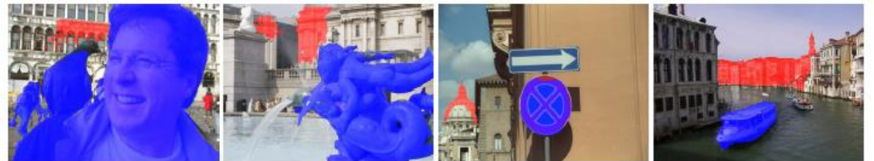
Figure 3: Examples of automatic ordinal labeling. Blue mask: foreground ( F_{ord} ) derived from semantic segmentation. Red mask: background ( B_{ord} ) derived from reconstructed depth.
